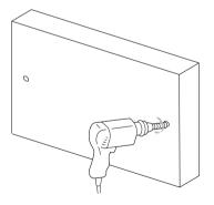
3 Secure 2 supplied screws in the holes, but leave 5mm between the screw head and the wall.
